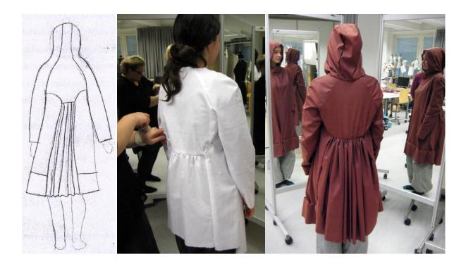
*Figure 11–13:* On the left, the design sketch for the back; in the middle, the trial garment of muslin; on the right, fitting of the garment with detachable felt lining. The overall process steps were design sketch, flat 1:1, trial garment, flat 1:1, design sketch, flat 1:1.
