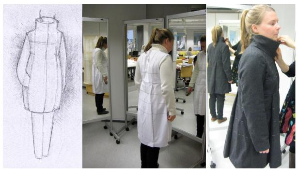
*Figure* 8–10: On the left, design sketch; in the middle, trial garment in muslin; on the right, fitting of the garment in wool. In the middle, the left-hand mirror shows the full-size flat pattern in the background. The overall process steps were design sketch, flat 1:4, flat 1:1, trial garment, draping 1:1, and flat 1:1.
