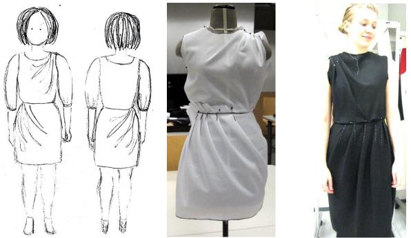
*Figure 26–28:* On the left, design sketch; in the middle, half-size flat pattern tested on model with muslin; on the right, fitting with wool crepe. The overall process steps were design sketch, flat 1:2 plus testing on model, flat 1:1, trial garment, and flat 1:1.
